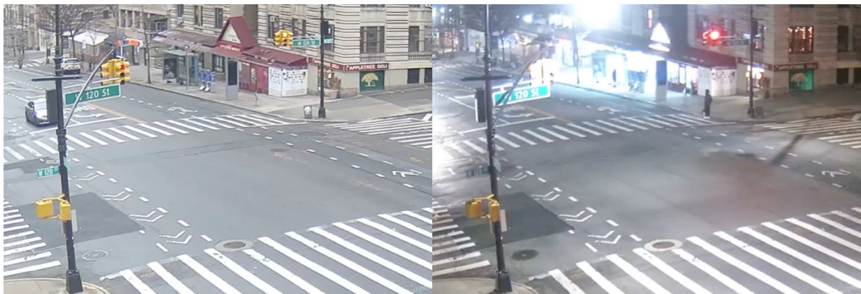
Figure 5 Video stream frames from day and night highlighting the challenge with traffic light status detection
