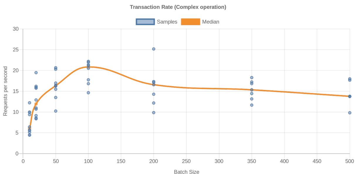
Figure 15: Transaction rate for complex transactions using WebSocket.
